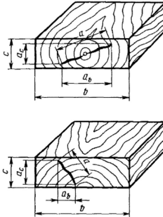
$$z_1 = \frac{a}{b} \text{ при } a_b > a_c; \quad z_2 = \frac{a}{c} \text{ при } a_c > a_b$$
